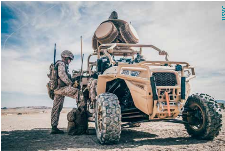
One of the first C-UAS systems operationally deployed was the LMADIS from Ascent Vision. Fit to Polaris MRZR light vehicles it integrates radar, electro-optics, electronic warfare, and Operator Assist (CUAS-OA) to detect, locate, track, classify, identify and neutralise small UAS.
