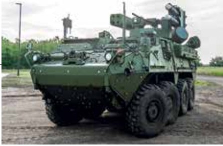
IM-SHORAD uses the Stryker 8x8 platform mounting the MOOG RlwP turret with a 30mm auto-cannon, Stinger ground-to-air missiles, and Longbow Hellfire antitank missiles. RADA Multi-mission Hemispherical Radar and a Wescam panoramic sight provide detection and fire control.
