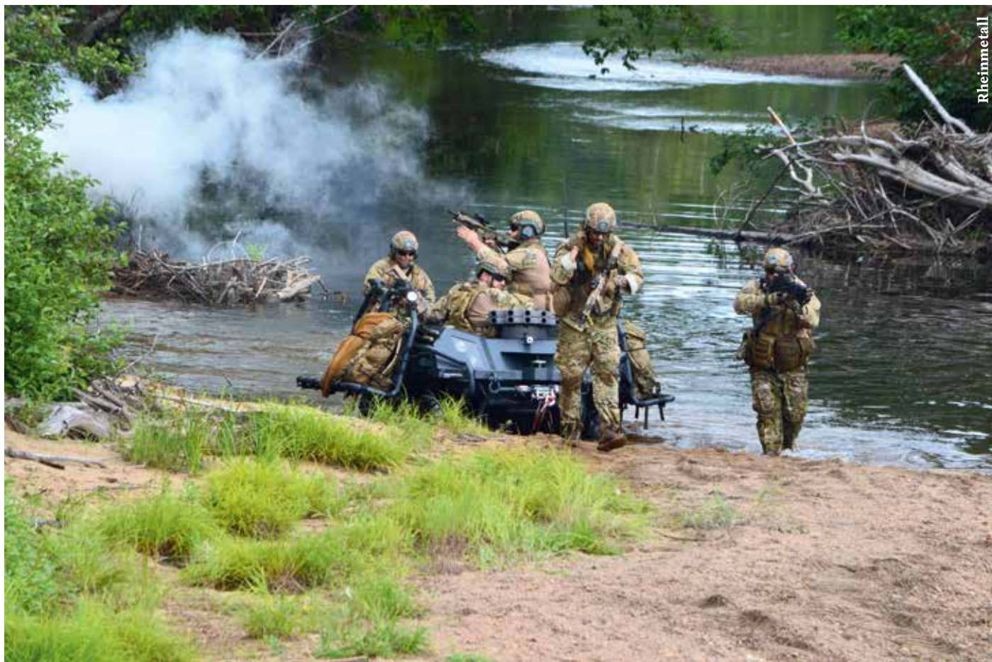
UGVs need to augment soldiers' capabilities to perform various tasks. Rheinmetall's Mission Master with its inherent swimming ability assists infantry to cross a water obstacle.
