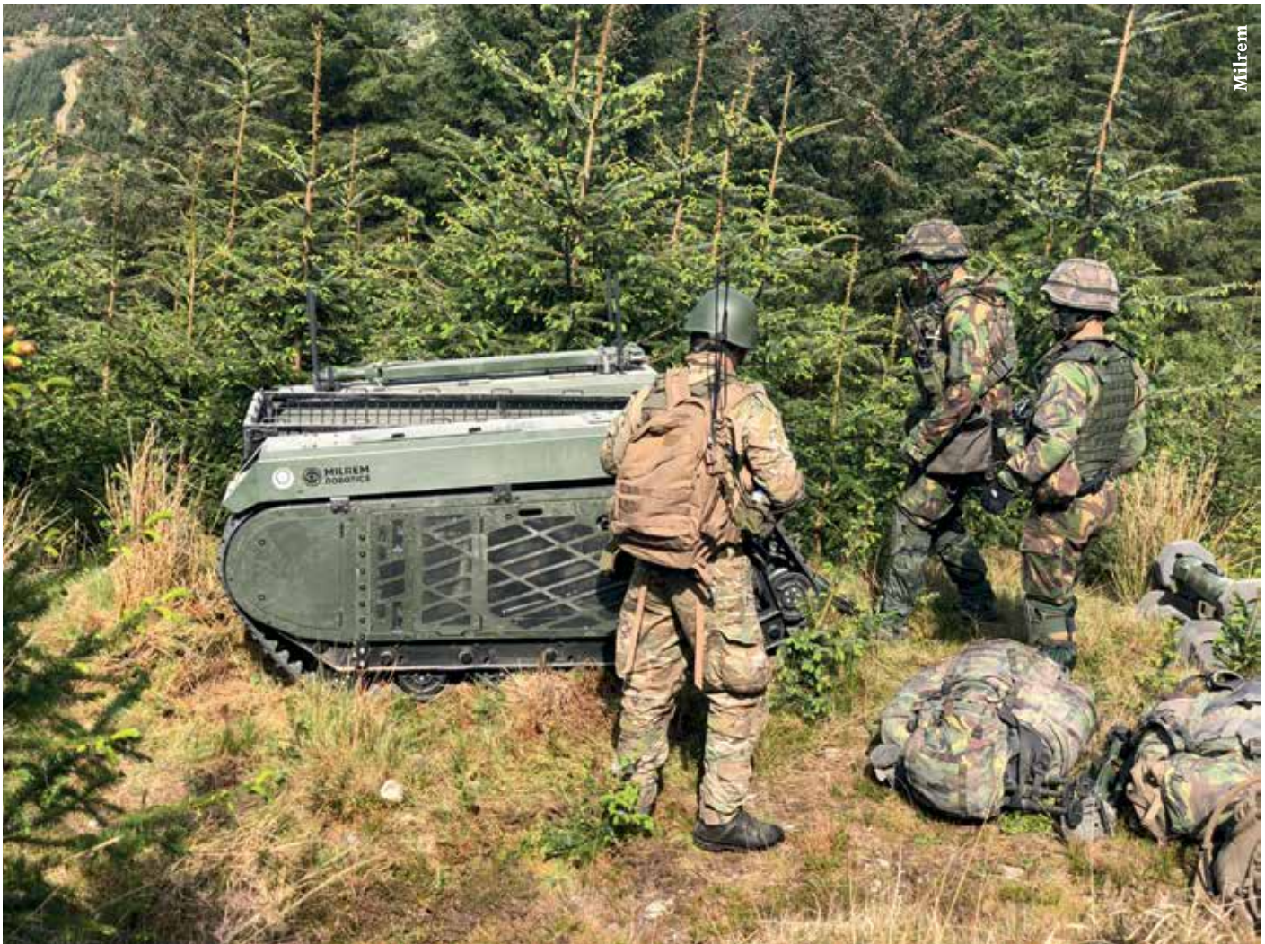
The Milrem THeMIS, here configured for infantry support, is designed to accept whatever attachments or systems a user requires which can be mounted to the frame.
