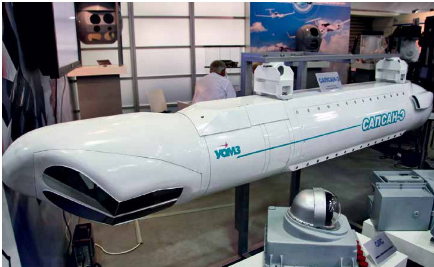
The Russian UOMZ Sapsan-E features several sensors including a low-light TV camera, anIRST / FLIR dual-band (IIR) sensor, a laser rangefinder and a laser designator.
