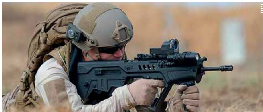
Israeli Weapons Industries (IWI) developed TAVOR feature bullpup design, is compact and offers various barrel lengths with minimal impact on its overall length.
