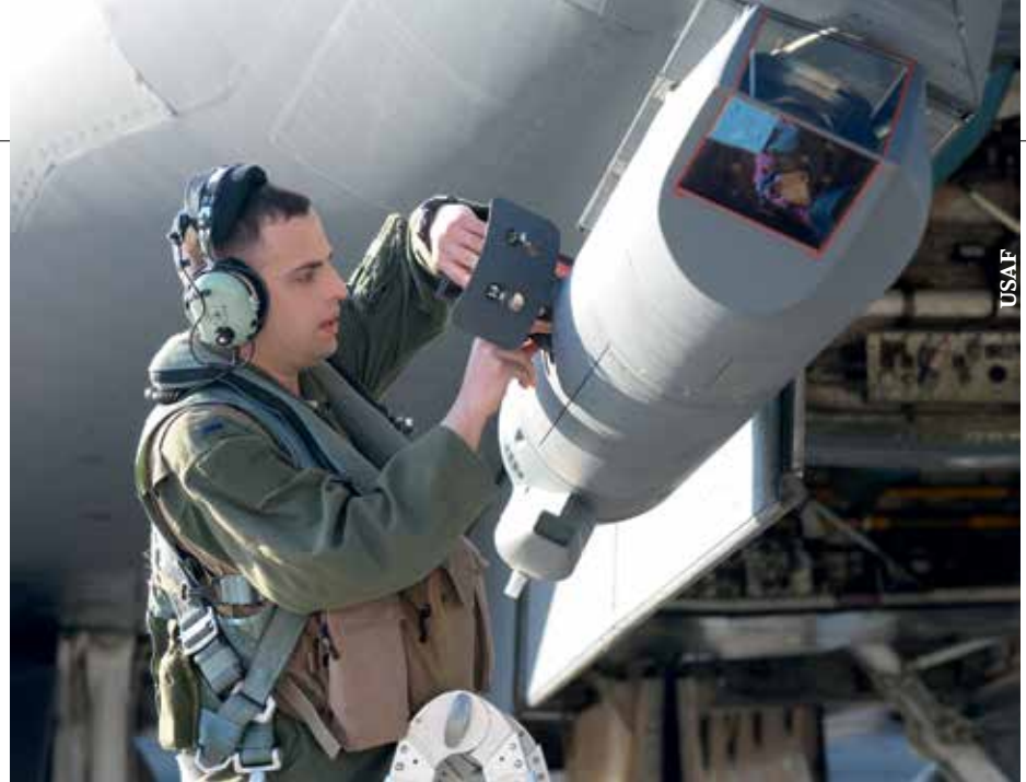
A B-1B Lancer bomber offensive systems officer loads software into a Sniper advanced targeting pod prior to a mission. The long-range targeting system provides aircrews with positive target identification, autonomous tracking coordinate generation and precise weapons guidance from extended standoff ranges.
