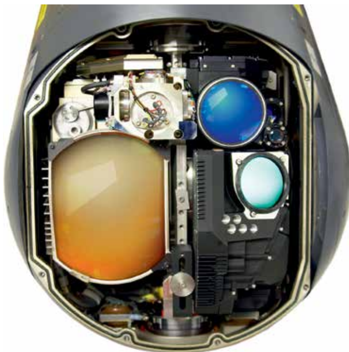
Northrop Grumman’s Litening pod includes a suite of advanced high-resolution sensors and a data link for intelligence, surveillance, reconnaissance (ISR) and target acquisition.
