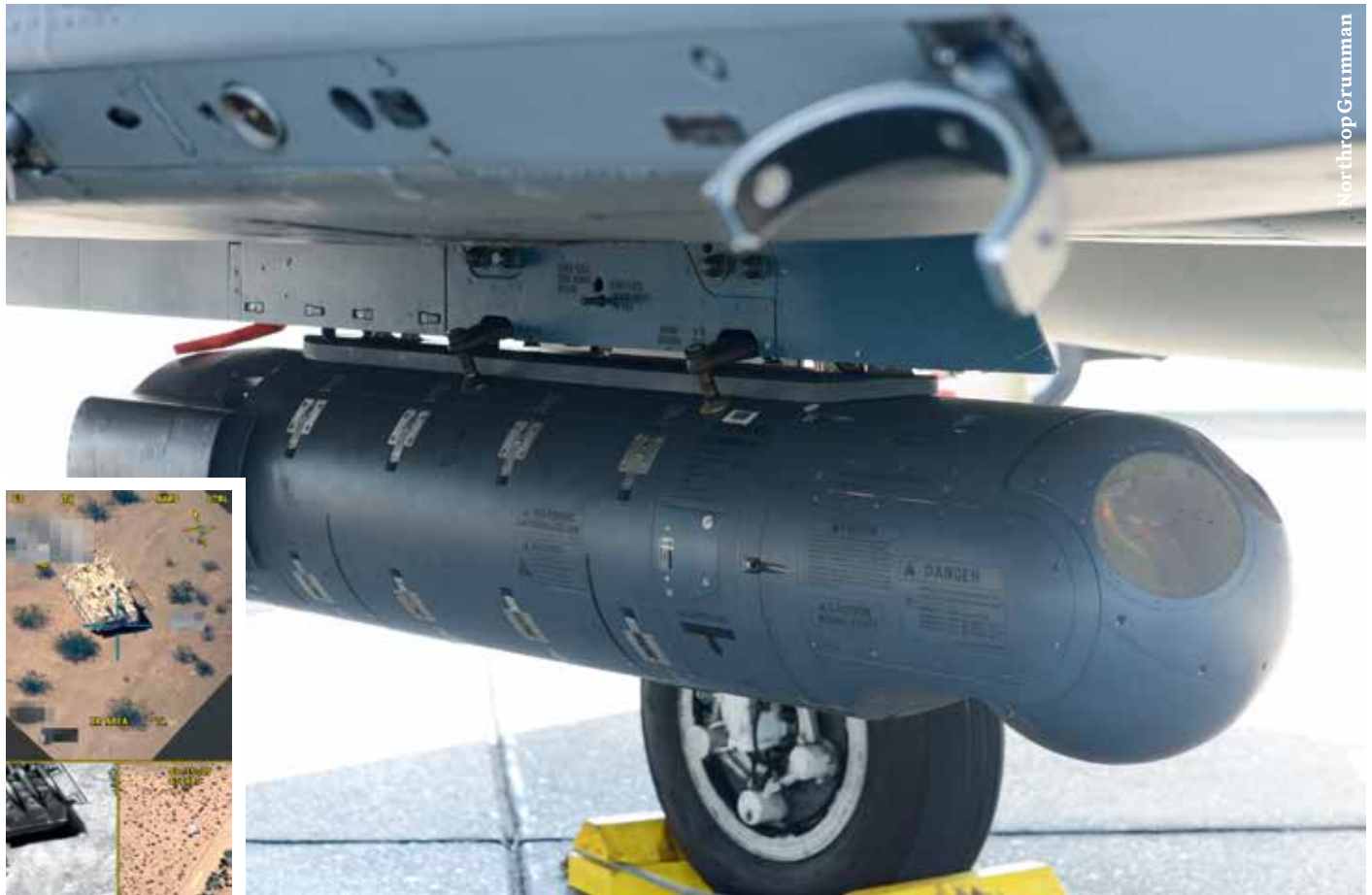
Northrop Grumman's Litening pod has seen over 20 years of service and has been integrated with a wide variety of aircraft. (Inset) Looking at the target via the Litening pod.
