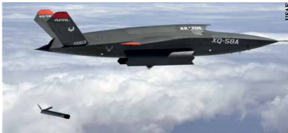
The Kratos XQ-58A Valkyrie has been used to release in flight a small Altius-600 UAV from its internal weapons bay.
