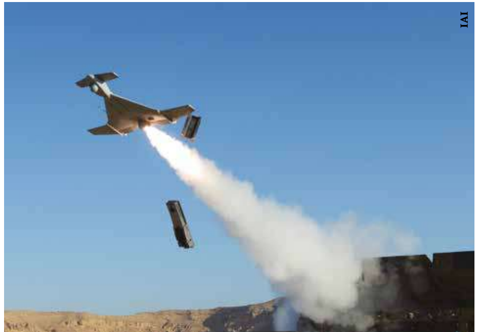
The IAI Harop was used by Azerbaijan's forces against the Armenian military, providing a persistent air threat due to its nine-hour endurance and anti-armour capability.
