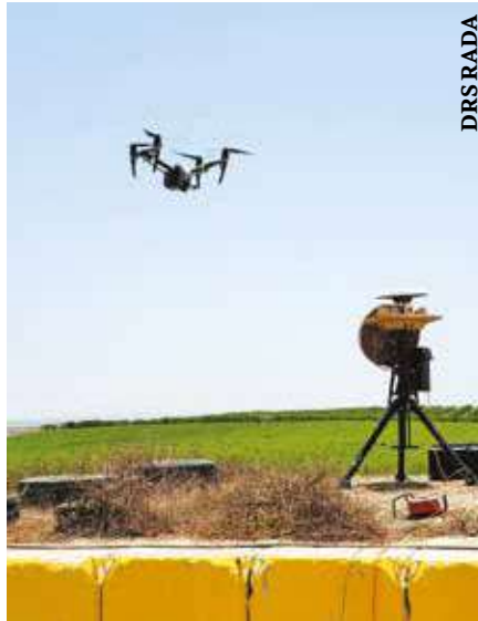
The ieMHR is a cutting-edge, ground-based, multi-mission radar for Counter-UAS, Very Short-Range Air Defense (VSHORAD), Counter Rocket, Artillery and Mortar (C-RAM), and Hemispheric Surveillance operational missions.
