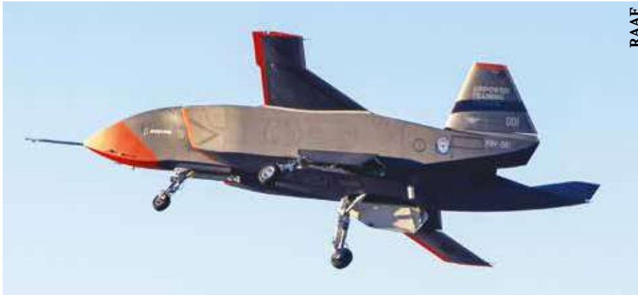
The MQ-28A Ghost Bat is being developed by Boeing Australia as a 'Loyal Wingman' for the Royal Australian Air Force.
