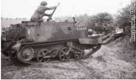
UGV forerunner - 2-inch mortar being fired from a Universal Carrier in Britain, 10 May 1943
