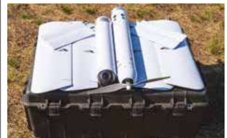
The Ukrainian developed Athlon Avia ST-35 Silent Thunder has an operational radius of 30km, a flight time of one hour and can carry a 3.5kg warhead.
