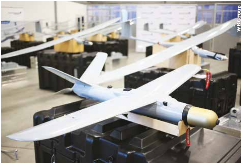
The WB Warmate is a self-contained, lightweight loitering munition with an operational radius of 30km and an operational speed of 50 miles per hour (80km/h). It can be deployed by a single user.
