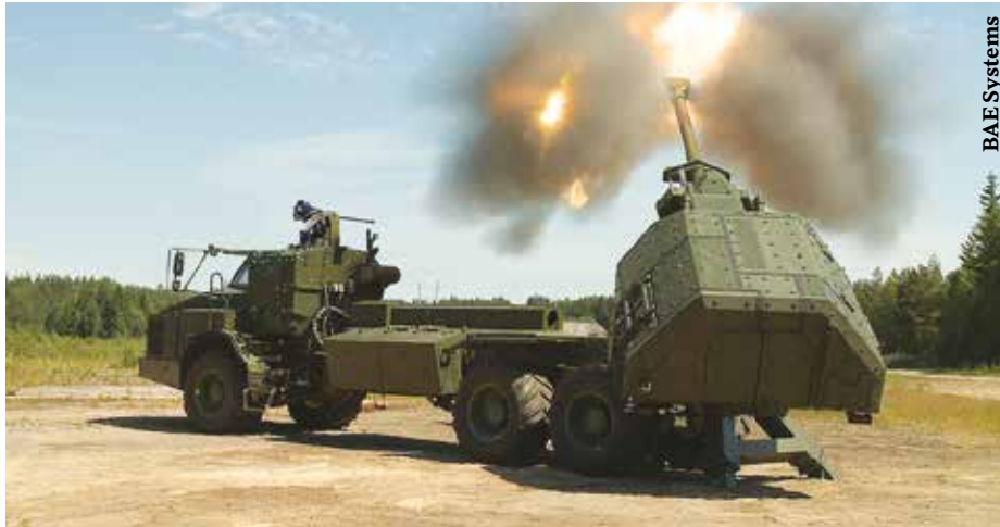
Sweden has supplied its BAE Systems Bofors Archer (6x6) 155mm SP artillery system to the Ukraine on the Volvo chassis.
