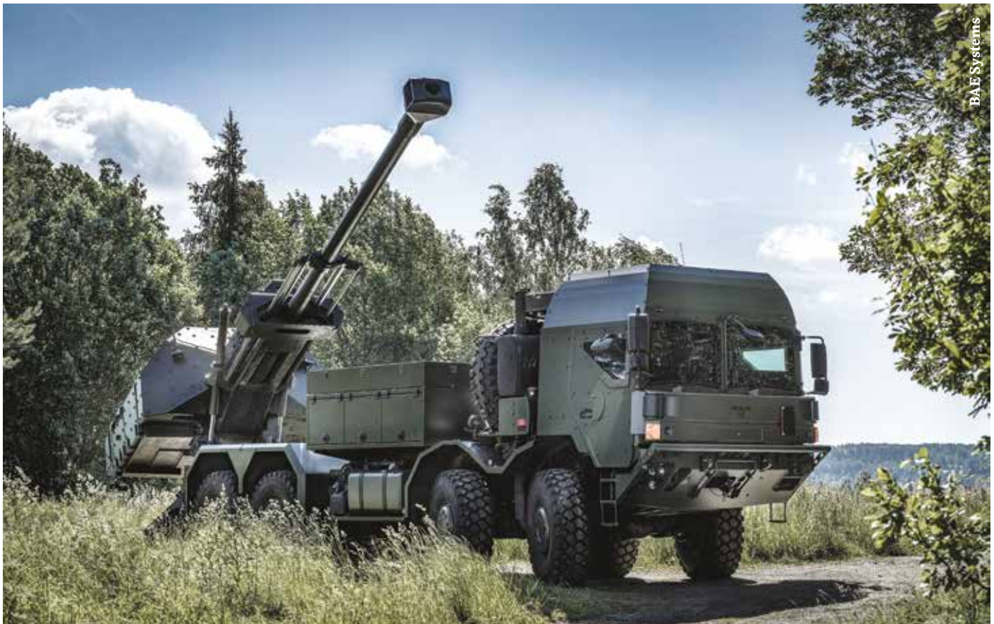
Future production BAE Systems Archer (6x6) 155mm system will be mounted on the Rheinmetall MAN Military Vehicles HX (8x8) cross country chassis.
