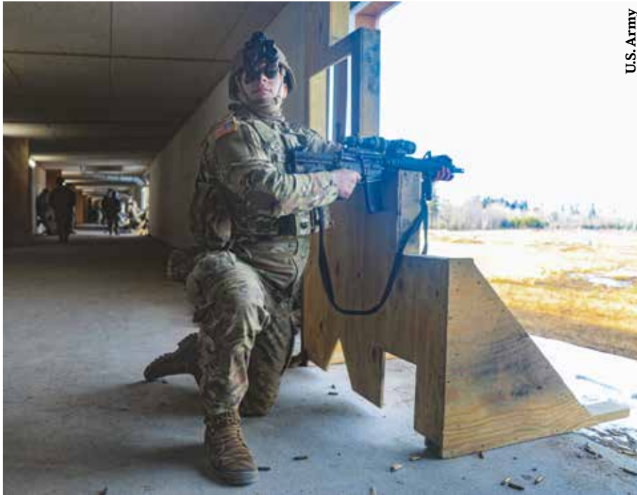
A soldier demonstrates the capability of the L3Harris ENVG-B by not having to look at the range directly to aim at his targets. The remote sight of the ENVG-B feeds its image to the advanced combat helmet mount, allowing the soldier to view their target without having to look at it.
