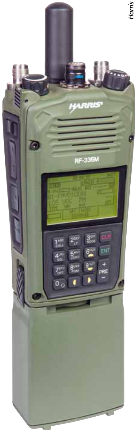
Software defined radios, such as this Harris RF-335M, are constantly improving in terms of being able to easily accept software updates to enhance their capabilities, much like the world of civilian communications and computing.
