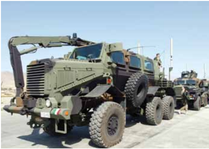
An Italian Army Buffalo; this Mrap is mostly used by route clearance parties as its hydraulic arm allows to inspect the road sides and culverts. (Armada/Paolo Valpolini)
