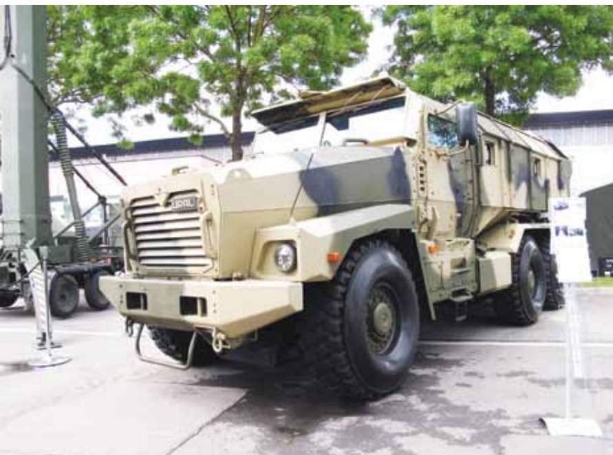
At Eurosatory 2012 Ural unveiled its mine-protected vehicle, based on the chassis of one of its 6x6 trucks. The Ural-ZA is obviously proposed for the Russian Army requirement. (Armada/Paolo Valpolini)
