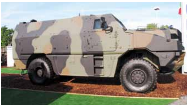
Born from a co-operation between Iveco DV and KMW of Germany the MPV is based on the Trakker truck chassis. The Italian Army will base most of its support vehicles on the MPV model. (Armada/Paolo Valpolini)
