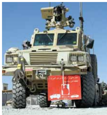
Canadian RG31 Nyala deployed to Afghanistan. This Mrap was developed by BAE Systems OMC and has been marketed and produced by both BAE Systems and GDLS. (Canadian DoD)
