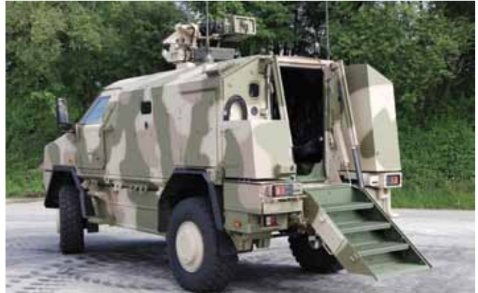
A rear view of KMW Dingo 2 HD. Given the height of the cabin floor, the rear powered ramp is fitted with steps. (KMW)
