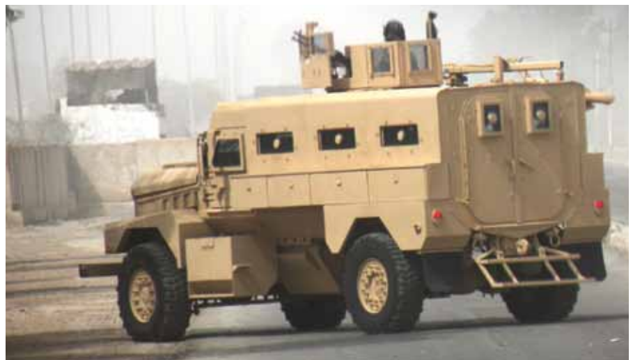
The Badger is the version of the Ilav acquired by the new Iraqi Army. The vehicle is a stretched variant of the Buffalo 4x4 and can carry up to 10 soldiers. (Armada/Paolo Valpolini)
