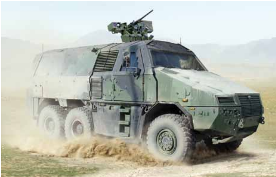
The KMW GFF4 is based on an Iveco Tracker chassis while the armoured cab is developed by KMW itself. The German Army is looking for a vehicle of more than 20 tonnes, which prompted KMW to propose its 6x6 MPV. (KMW)
