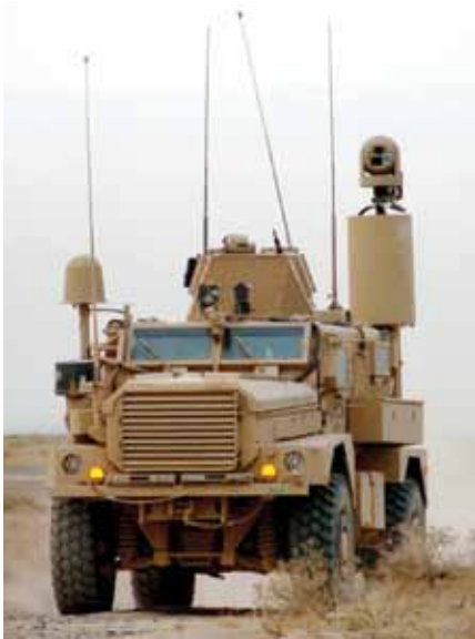
The US Marines Corp has been the launch customer for the Cougar and is one of the major users of the 4x4 version, here equipped with an ISTAR system. (US Marines Corp)
