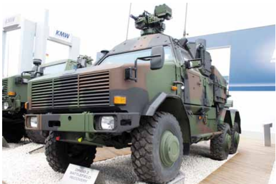
The Dingo has been developed in numerous variants. Featured here the battlefield recovery vehicle based on the Dingo 2. (Armada/Paolo Valpolini)
