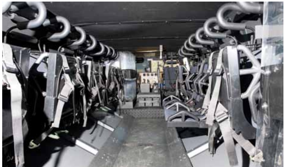
This inside view of the Renault Trucks Defense Higuard clearly reveals the energy absorbing folding seats that were adopted to accommodate ten dismounts in the rear compartment. (RTD)
