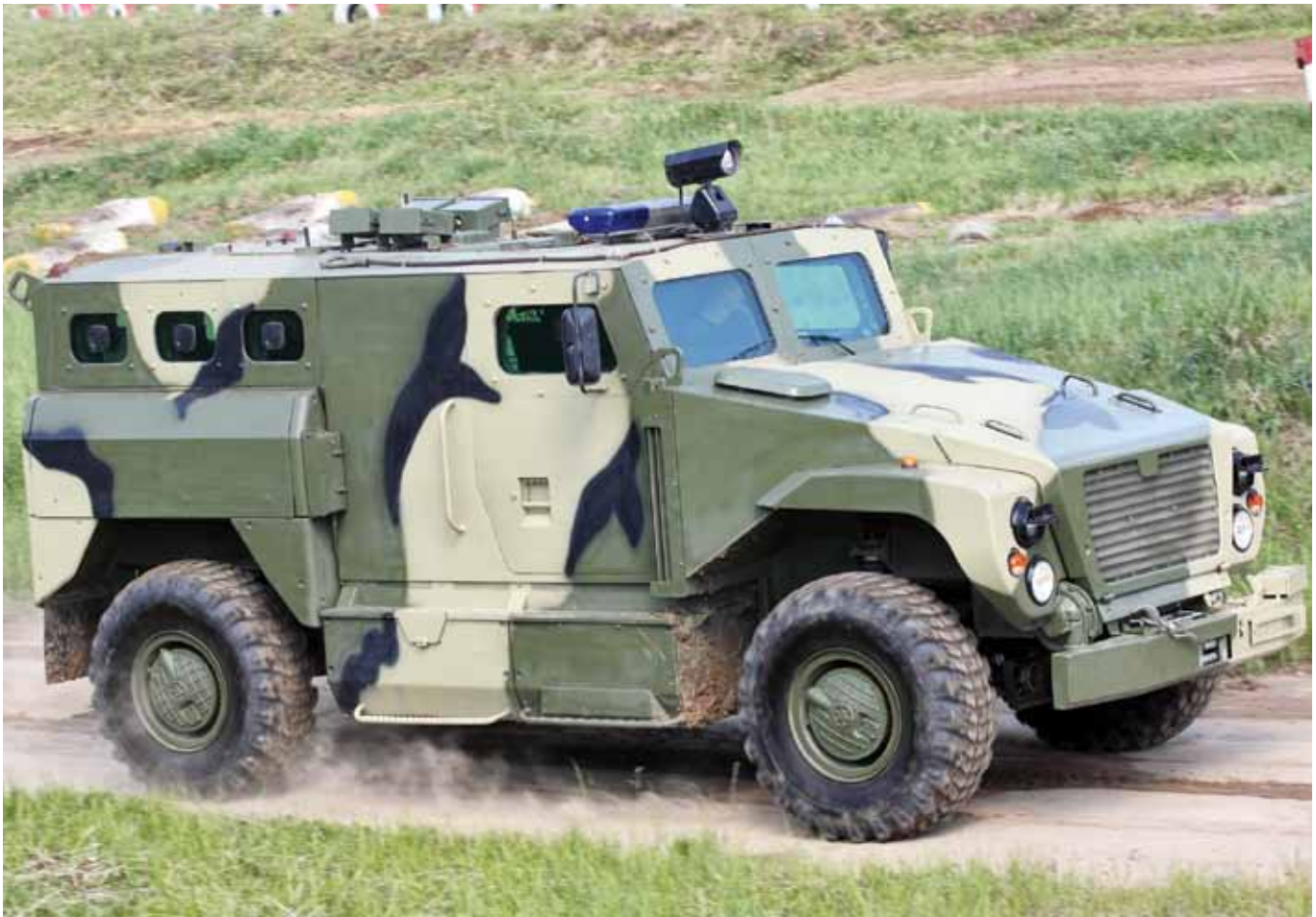
With eyes set on a potential lucrative Russian Army contract, Arzamas developed the SPM-3. It is probably the lightest mine-protected vehicle proposed to the services by the Russian industry. (V. Kuzmin)
