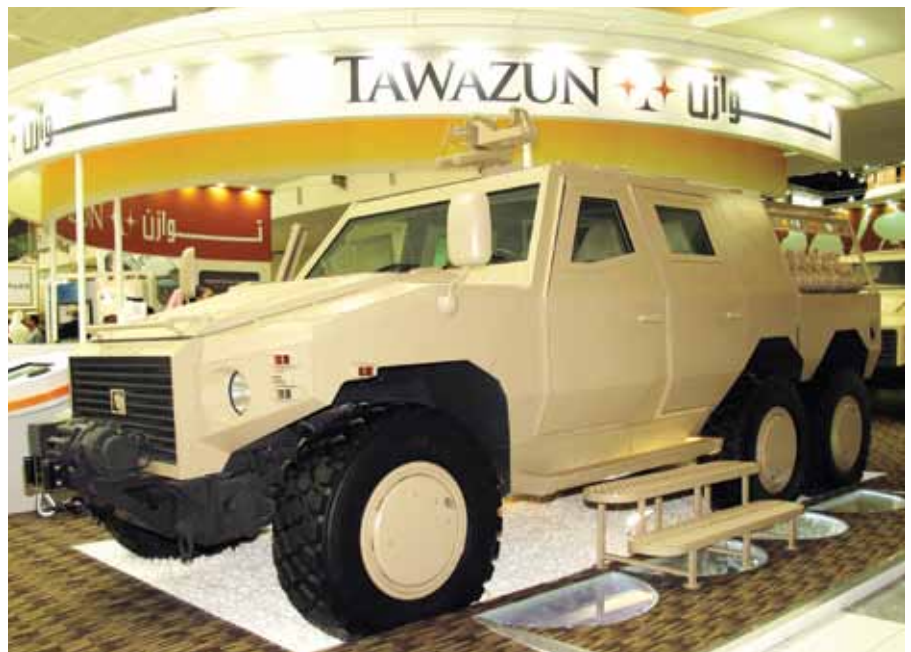
Among the many versions of the Nimr the 6x6 configuration features a highly protected ensemble that is definitely part of the MPV category. (Armada/Paolo Valpolini)
