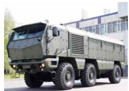
One of the latest nations in search of a mine-protected vehicle is Russia. Kamaz answered this requirement with the Typhoon mine protected truck that can host up to 18 soldiers. (Kamaz)
