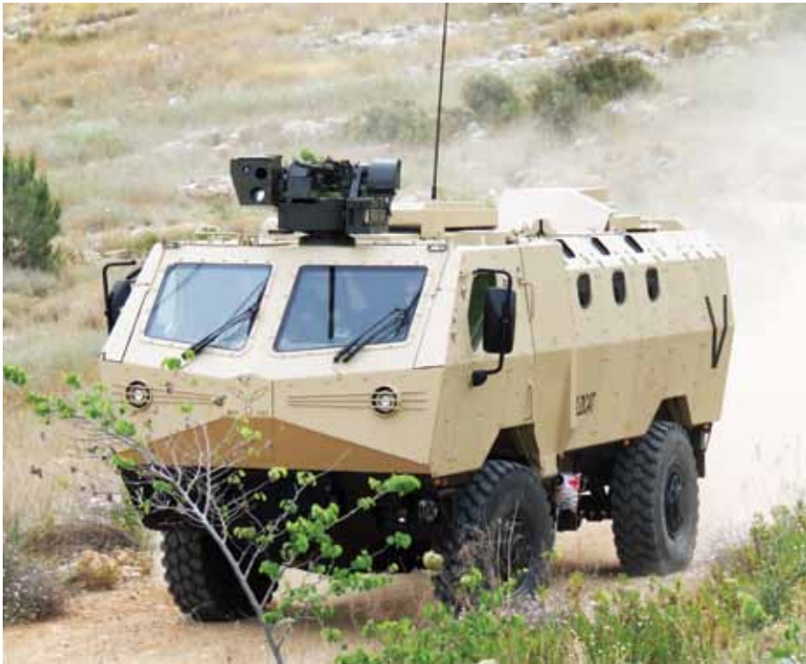
The IMI Wildcat is based on a Tatra 4x4 truck chassis. The marketing campaign carried out by the Israeli company also includes leasing solutions. (IMI)
