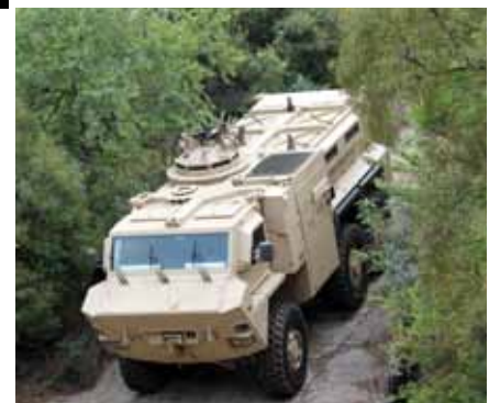
The RG35 6x6 together with the smaller 4x4 variant are ready for production, featuring as they do an 80% parts commonality. (BAE Systems)
