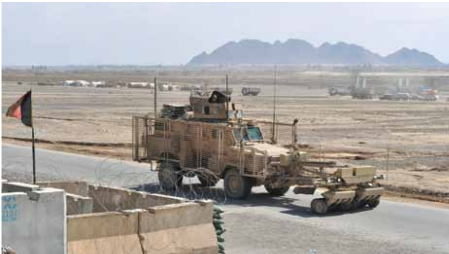
A Canadian 4x4 Cougar equipped with mine rollers and bar armour. The Cougar has become a GDLS product following the acquisition of Force Protection. (Canadian DoD)
