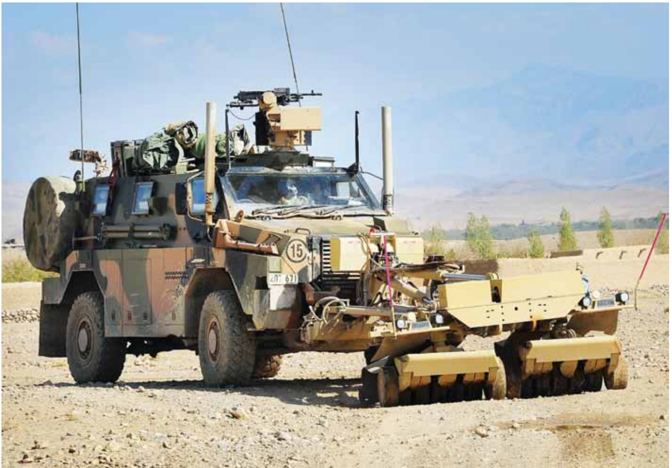
The Bushmaster, designed and produced by Thales Australia, here equipped with mine rollers, is a lifesaver in Afghanistan for Aussie soldiers. (Australian MoD)
