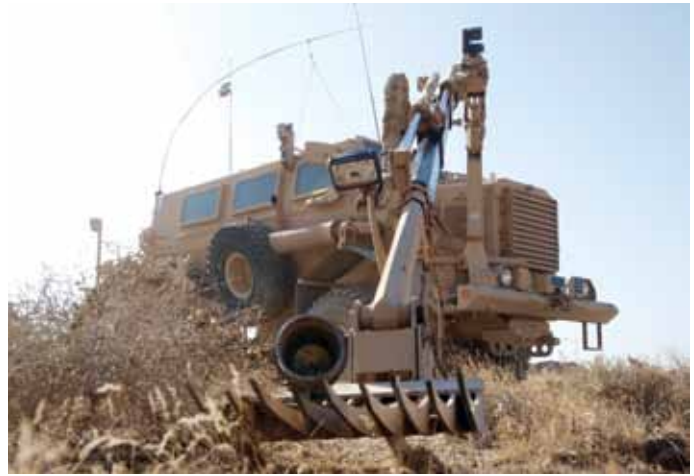
To further decouple the operators from any possible threat GDLS has launched a new version of the Buffalo that in the medium term will become a robot control platform. (Armada/Paolo Valpolini)
