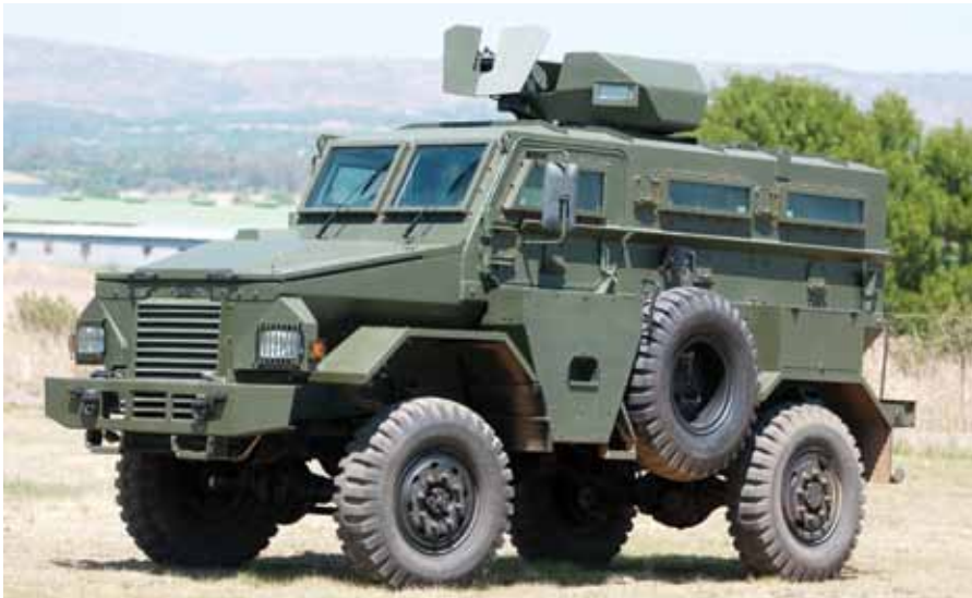
OTT of South Africa developed an all-terrain MPV based on a Tata 4x4 chassis; known as M26 it is in service with the Kenyan Army in the M26-15 version. (OTT)
