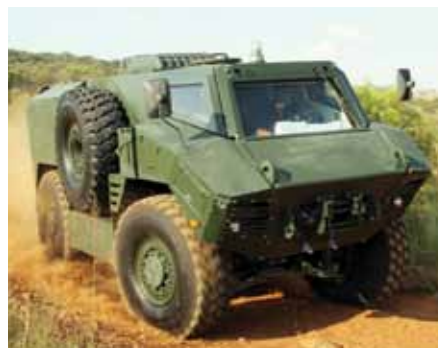
The 4x4 version of the RG35, unveiled in 2011 and also known as the RPU for Reconnaissance, Patrol, Utility, was developed to take part in the Canadian TAPV bid. (BAE Systems)
