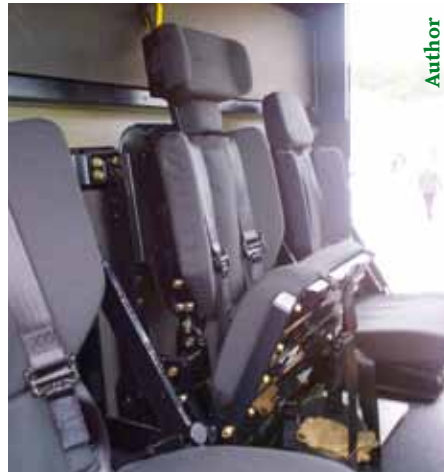
Blast resistant/shock absorbing seats (these troop seats are in the latest US Marine Corps AAV7) have been shown to significantly reduce injury to soldiers.
