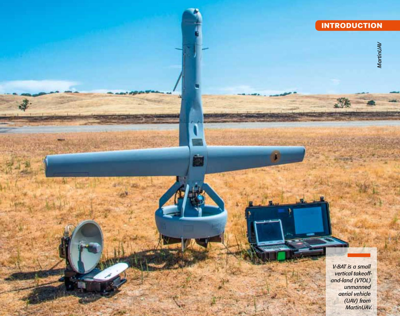
*V-BAT is a small vertical takeoff-and-land (VTOL) unmanned aerial vehicle (UAV) from MartinUAV.*
