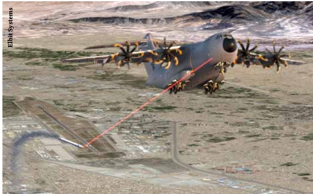
This artist's concept show an A400M equipped with J-MUSIC defeating a ground-launched SAM
