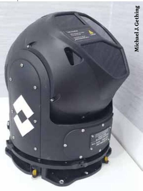
The UltraForce 275-HD EO/IR sensor turret is ITAR-free and repackaged for footprint-constrained platforms.
